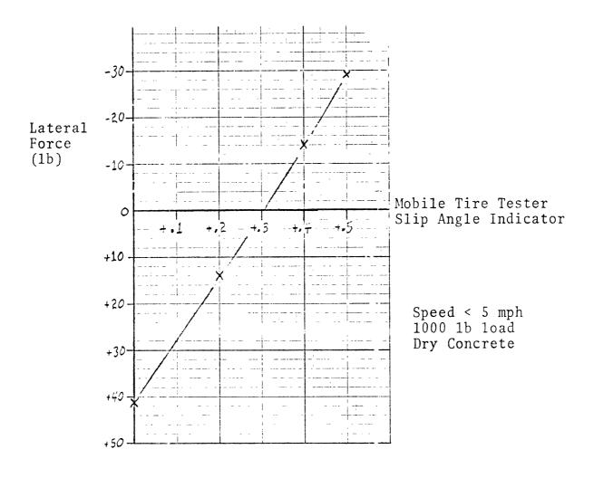
Figure 1. Calibration of the mobile tire tester slip angle indicator using a certified zero lateral force tire from Ford Motor Company.
