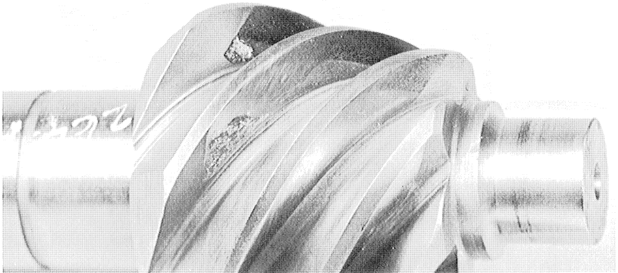
Figure 28. Pitting of hypoid pinion.
