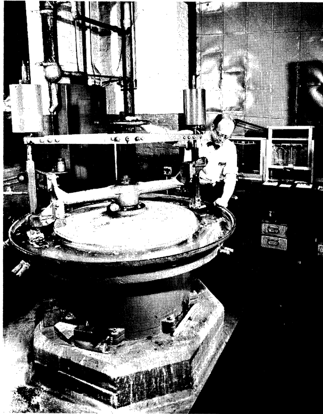
Figure 9. Apparatus for abrasion testing in a gritty environment.
