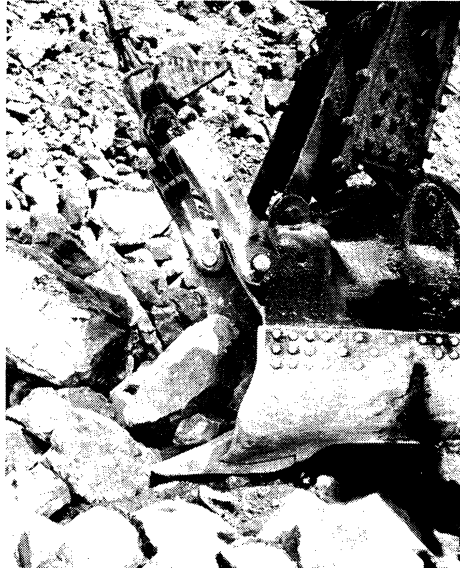
Figure 8. Power shovel bucket digging in rocks and boulders. The wear situation provides gouging abrasion and considerable impact. Both are associated with high stresses and require tough alloys to withstand them. Austenitic manganese steel is usually the preferred material.
