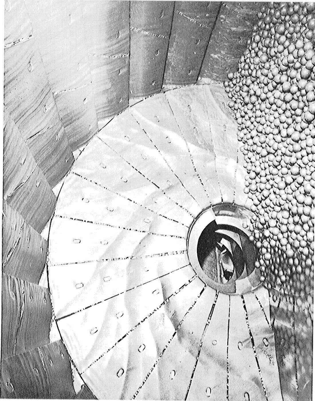
Figure 2. Interior view of a 13 foot diameter ball mill showing partially worn end and shell liners.
