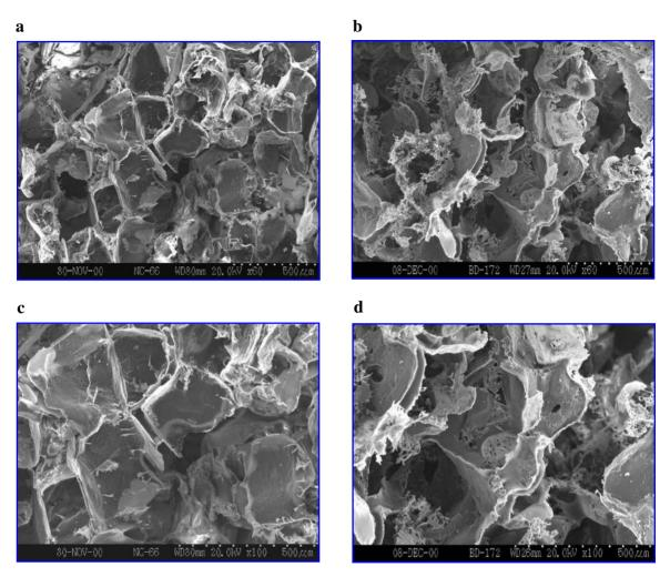
**FIG. 5.** Electron micrographs of the cross-section of gas foamed polymer scaffolds prepared using the salt fusion process. One hour of salt fusion results in the presence of a few very small holes in pore walls (a,c) similar to those in the solvent cast scaffolds. The 24-h salt fused scaffolds display a disorganized pore structure in which adjacent pores seem to feed into each other (b,d).
