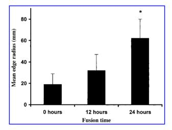
**FIG. 4.** Increase in the radius of curvature of salt crystal edges prior to addition of polymer in the solvent casting/particulate leaching method. Radii were measured from electron micrographs of salt crystals fused for 0, 12, and 24 h. Based on an ANOVA followed by comparisons between group means (Bonferroni *t* tests), the change in mean edge radius from 0 to 12 h was not significant (p > 0.05); however, the change from 12 h to 24 h was extremely significant (p < 0.001).
