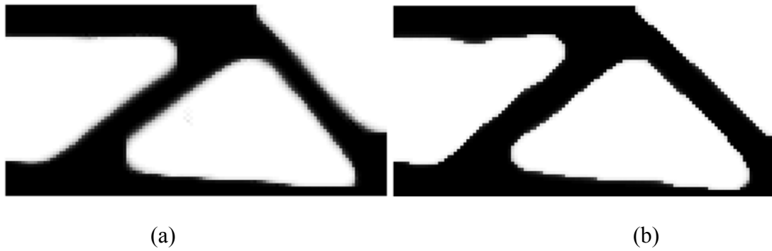
Figure 2.3.2. Design results of cantilever beam with perimeter constraint and additional density penalization ( w_\rho is set to 1000). (a) TV_2 (P_u=5) , (b) TV_4 (P_u=5)
