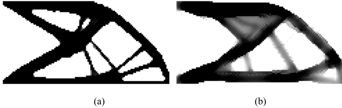
Figure 2.3.7. Design results of cantilever beam with MOLE constraint ( \varepsilon_r=0.01 , \varepsilon=0.1 , p=4 ). (a) r=1 and (b) r=3
