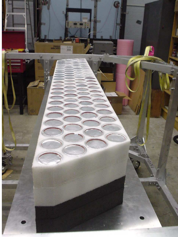
Figure 5.8: The array of crystal/PMT assemblies in the CREST-I instrument. These crystals were covered by thin aluminum caps.
