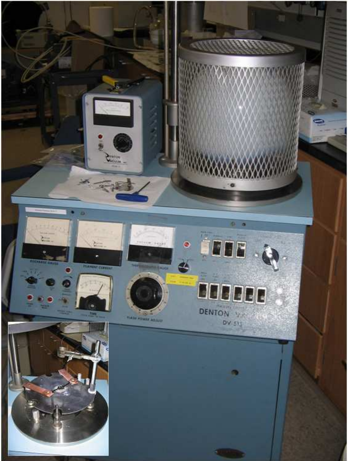
Figure 4.24: Pictures of the vacuum evaporator and the evaporation table/supporting structures inside the glass dome in the inset at bottom-left.
