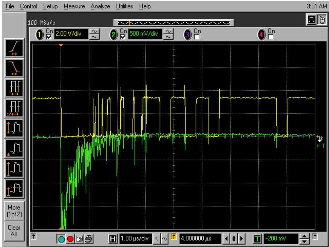
Figure 4.28: The discriminator output observed on the screen of the oscilloscope with a latch time of 400 ns. Channel 0 in yellow shows the discriminator response from the BaF 2 /PMT crystal output induced by atmospheric muons (equivalent to \sim 3 MeV) for the signal for channel 1 shown in green. For ease of observation, these signals are boosted by factors of 2.5\times and 10\times at the output and the input of the discriminator respectively.
