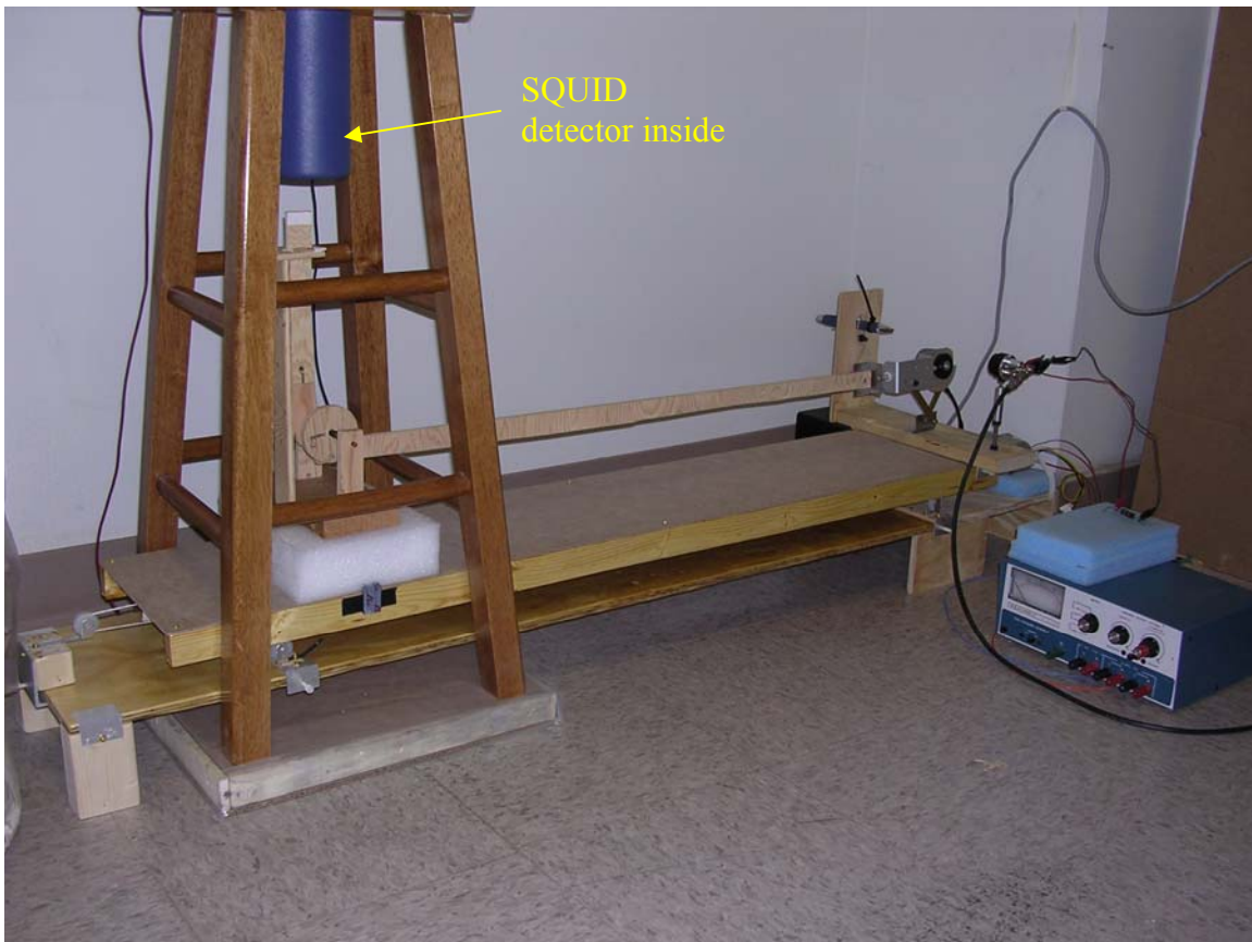
Figure 2.1 Picture of the remanence measurement-base SQUID imaging system with 1D scanning ability.
