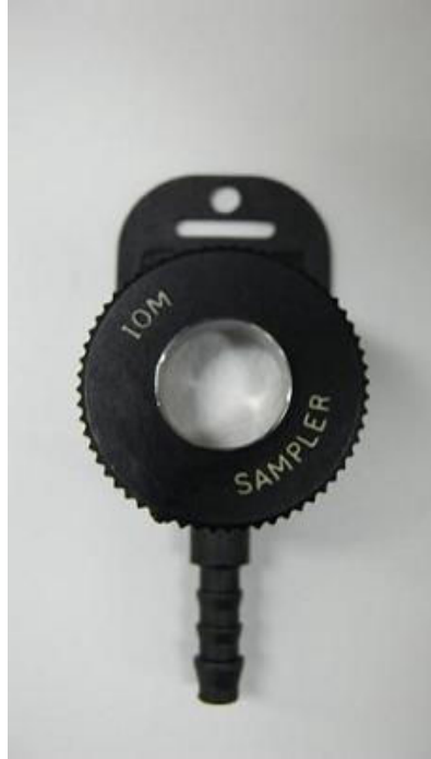
Figure 5.8 IOM sampler used to collect the inhalable aerosol particle size fraction, shown with the stainless steel cassette in place.
