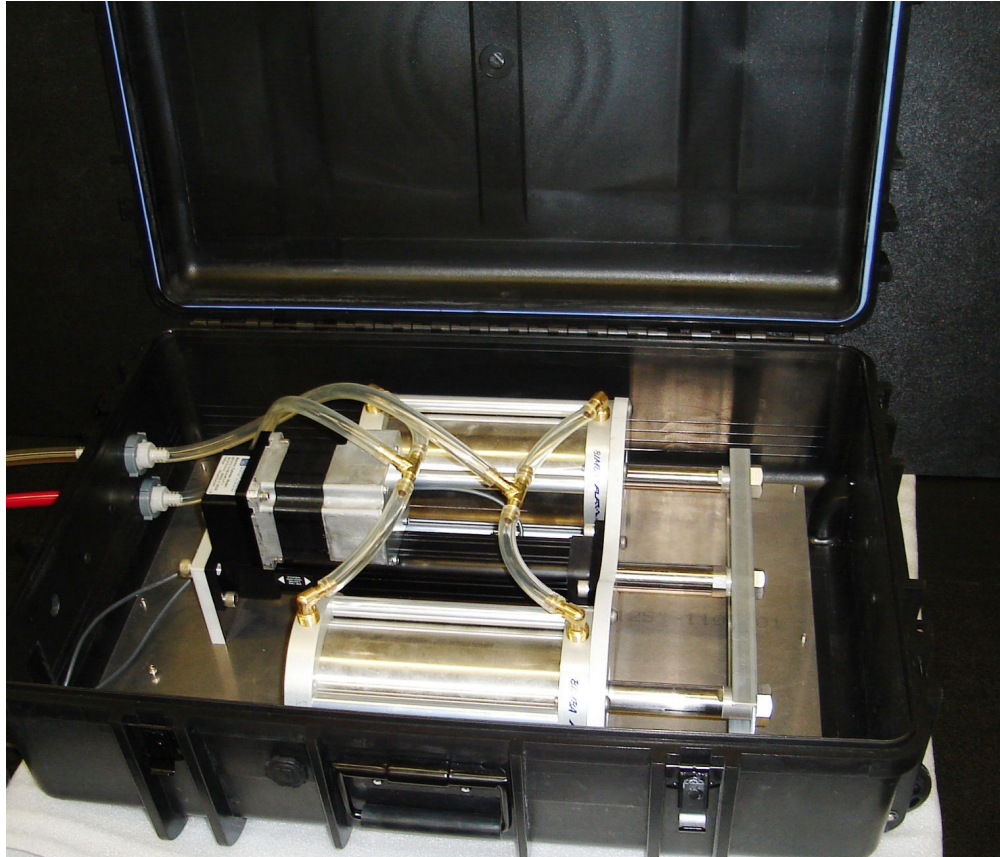
Figure 6.10 Mannequin breathing machine, consisting of two pneumatic cylinders and a servo-linear actuator that cycles in and out to produce a representative range of human breathing flowrates.
