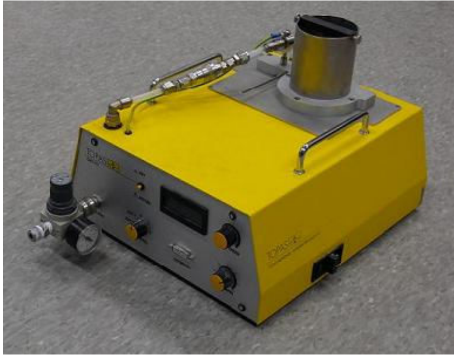
Figure 6.5 One of the Topas dust generators used to aerosolize and inject narrowly graded powders of fused alumina into the wind tunnel.
