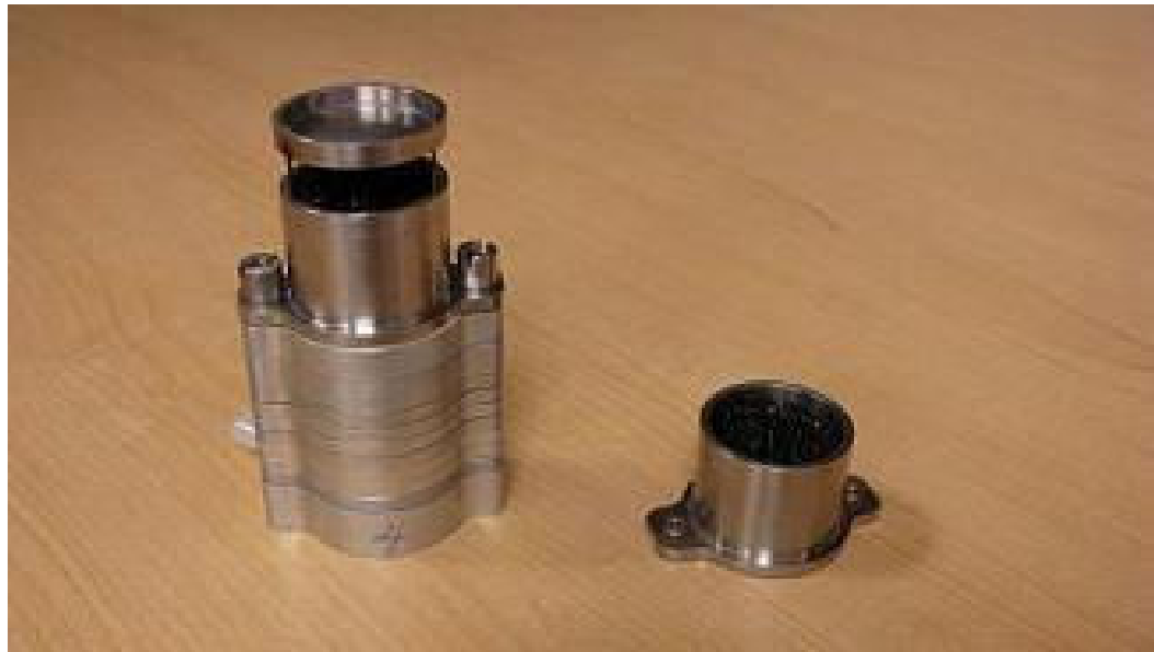
Figure 6.8 Modified Marple-type cascade impactor used to measure particle size distributions, shown assembled with the cap (not used here). Also shown is one of the disassembled top foam stages.
