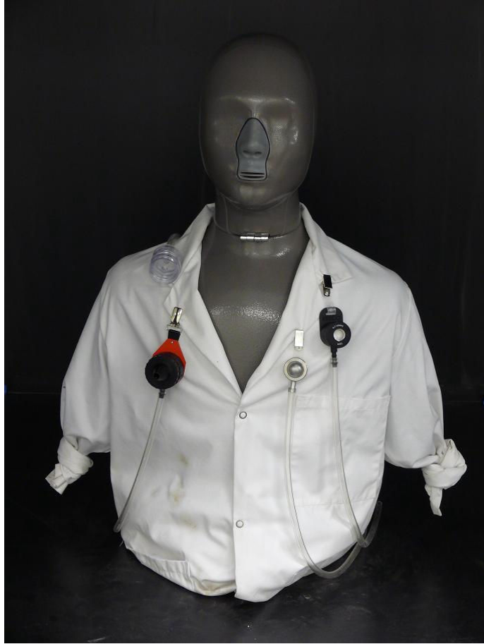
Figure 9.1 Experimental set-up for assessing personal sampler performance at ultra-low windspeeds, showing the mannequin with all four personal samplers tested. Not shown is the bag situated on the back of the mannequin torso that held the four sampling pumps.
