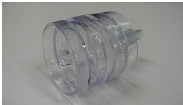
Figure 5.7 Plastic 37-mm cassettes used for aerosol sampling that can be operated in either the (a) open-face or (b) closed-face configuration.
