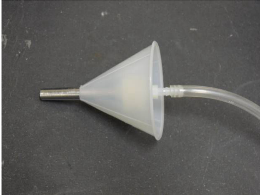
Figure 8.1 Isokinetic reference sampler, shown with plastic conical piece and pump tubing, which was used to measure the actual aerosol concentration inside the wind tunnel.
