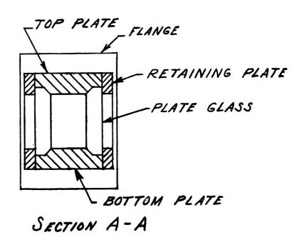
FIG. 1 - SHOCK TUBE TEST SECTION
