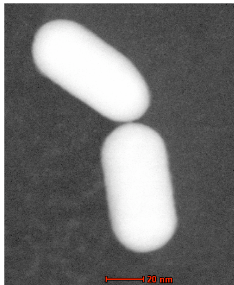
Figure 4.5: Dimer 2; angle dipole with separation \sim 1 nm.
