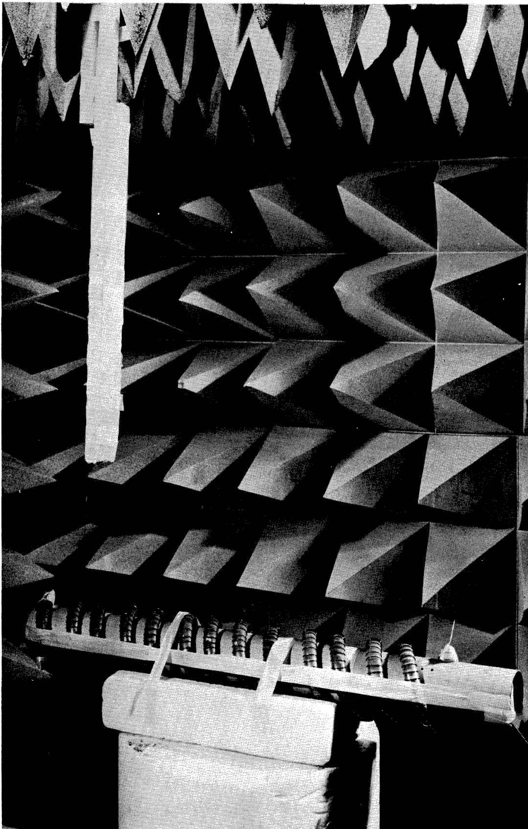
FIG. 2-30: ANTENNA 232, A BIFILAR HELIX ANTENNA WITH A FERRITE FILLED HELICAL WINDING SHOWING THE LOCATION OF THE LOOP PROBE WITH RESPECT TO ANTENNA 232.
