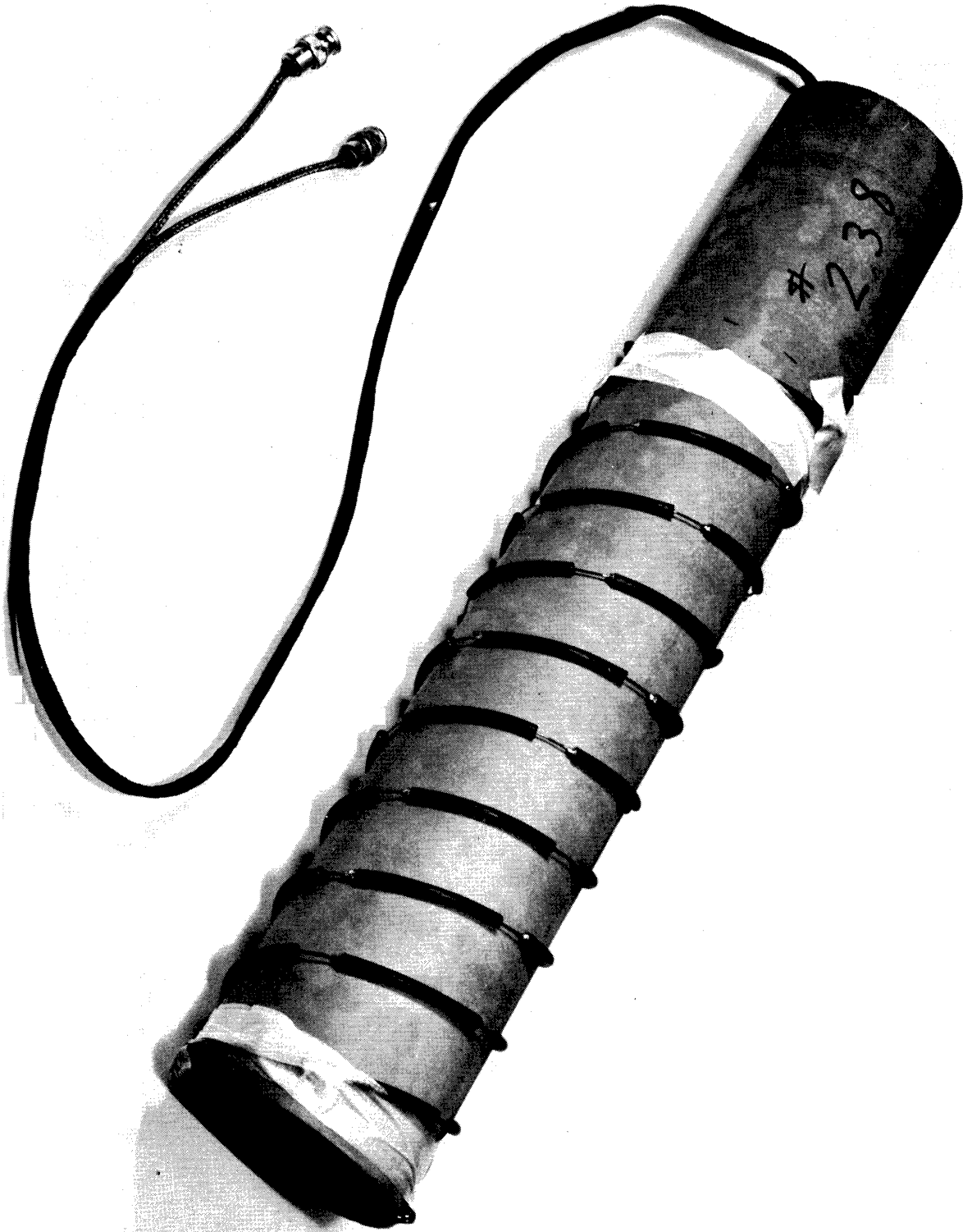
-31: ANTENNA 238, A BIFILAR HELIX ANTENNA WITH SHORTED TRANSMISSION INDUCTORS USED AS LOADING.
