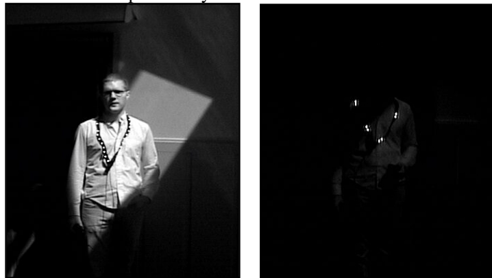
Fig. 8. IR views of old vs. new necklaces in direct sunlight
