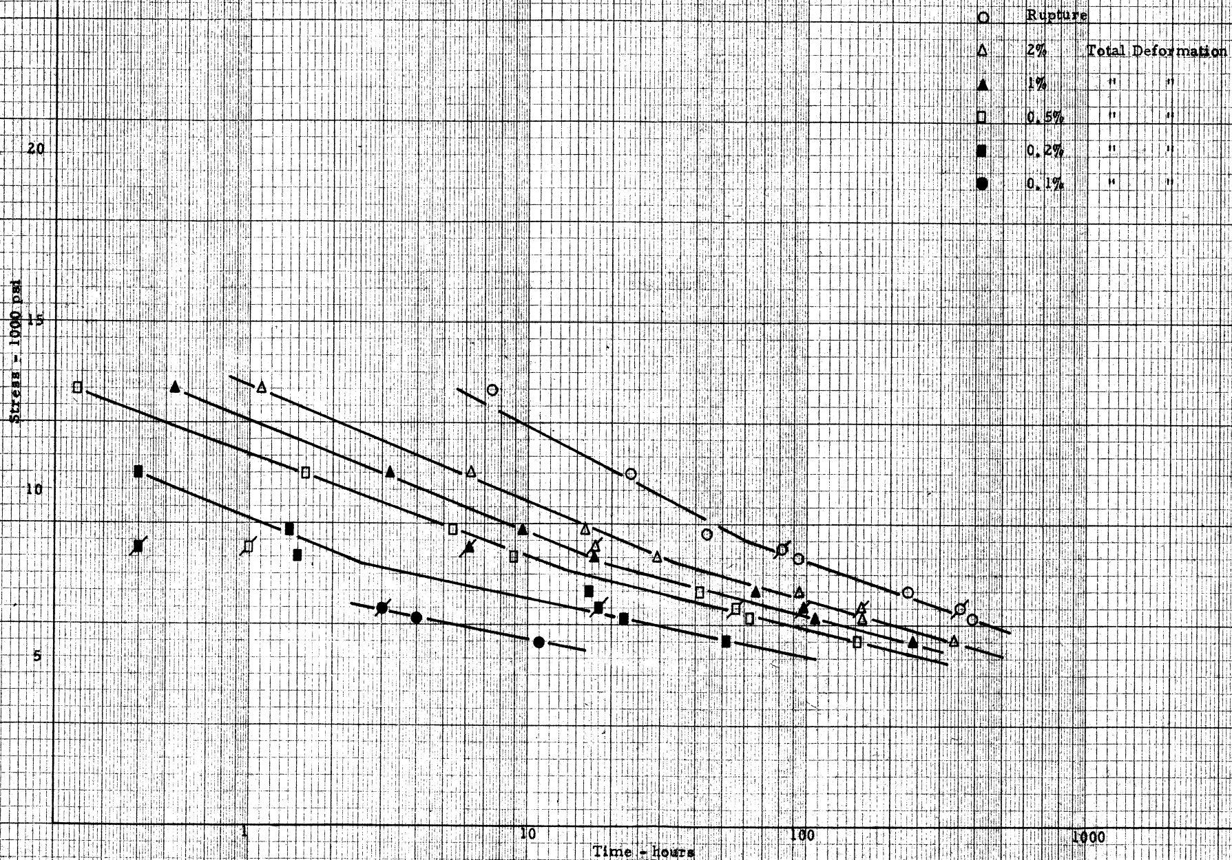
Figure 5. - Stress-rupture and stress-total deformation time curves obtained at 1650°F for sheet specimens of Hastelloy X, Heat X1037.
