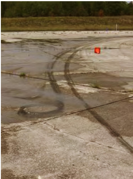
Fig. 6: Skid marks from the first rollover of the unit truck
