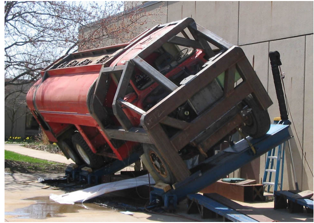
Fig. 2: The unit truck with roll bars on the UMTRI tilt table
