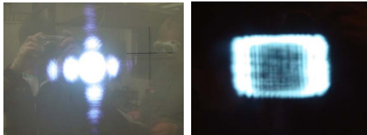
Figure 2-5: Far field and near field beam shape of TRW DP-11
