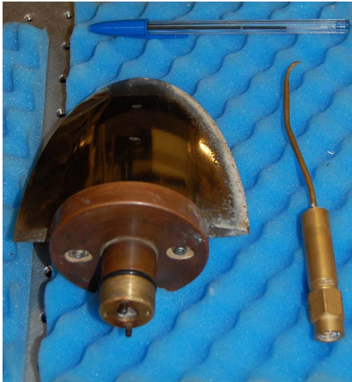
Figure 4-9: Simulated injection hole for polymer characterization (right) and actual hydrofoil (left)
