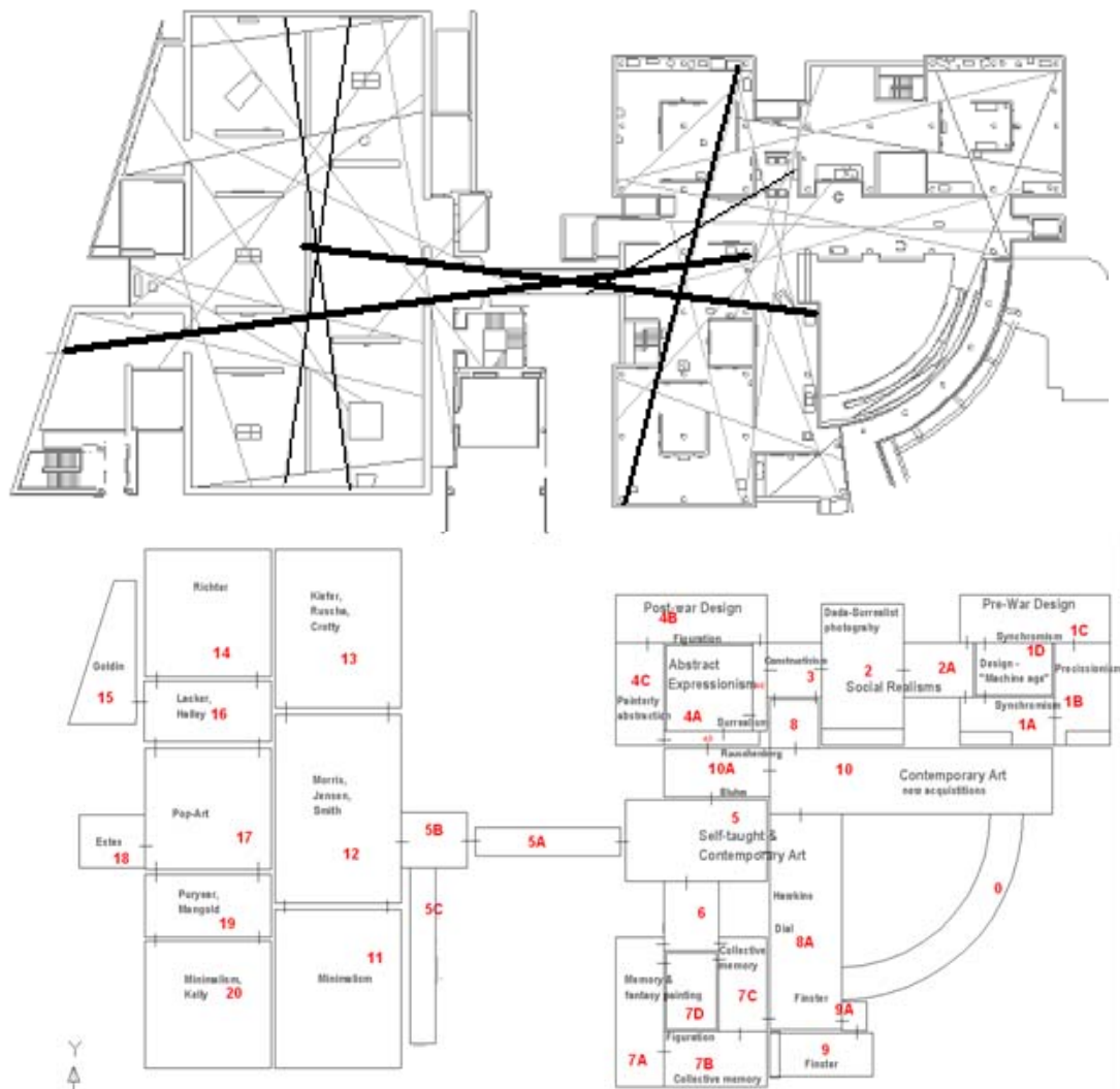
Figure 6.30 Comparison of axial line analysis and narrative organization within the convex map
