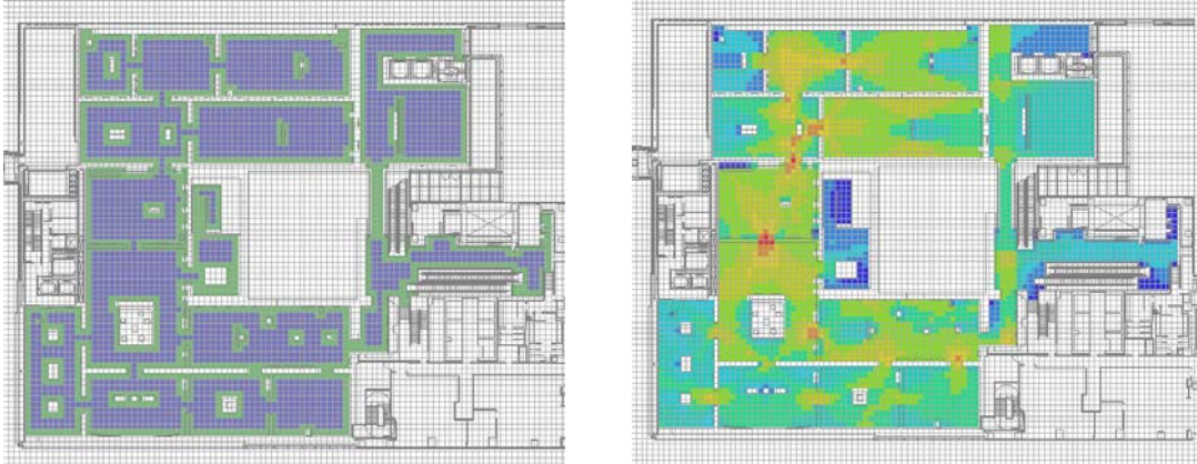
Figure 3.7 Steps of generating visibility graph analysis in Depthmap ; setting the grid and selecting the paces where the graph will be generated ( left ); and visual connectivity graph ( right ).
