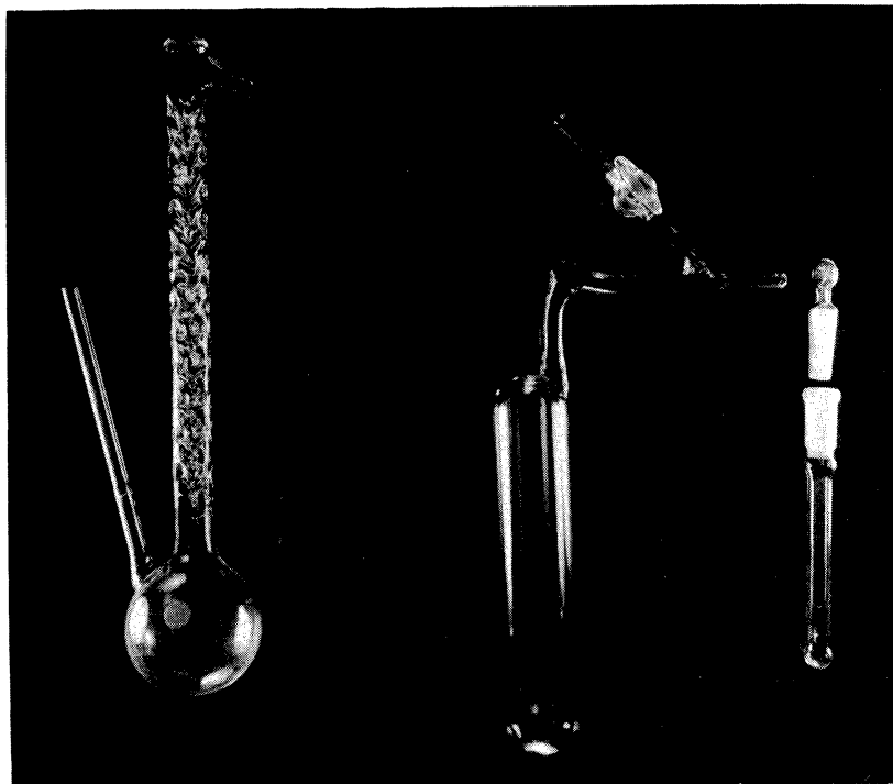
Fig. 17. Glass apparatus for vacuum distillation of styrene, and glass-stoppered tube for irradiation and polymerization of styrene.
