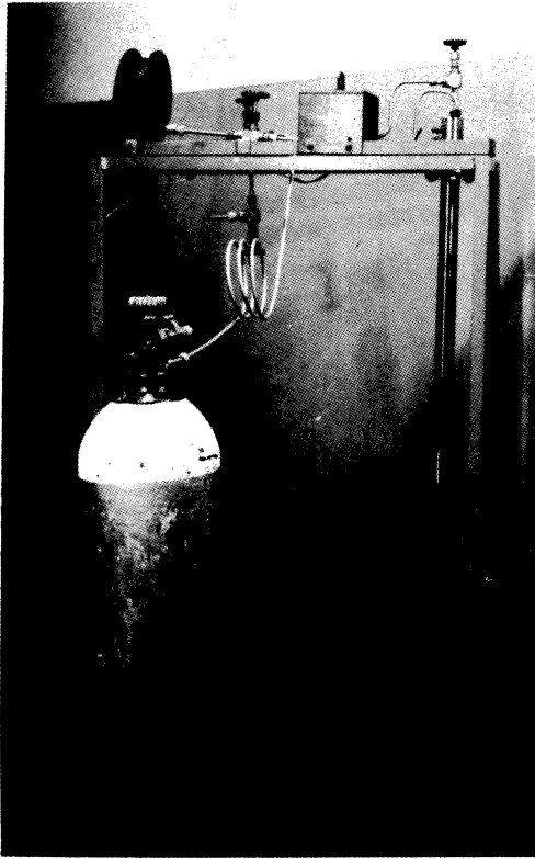
Fig. 55. Pressure Reactor in Rack and Connected to High Pressure Gas Cylinder.
