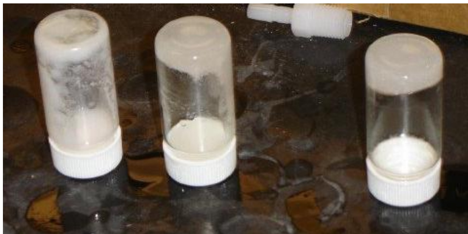
Figure 3.4: Pour point samples. The gel in the vial on the left was easily broken down upon inversion of the vial. The gel in the vial in the middle was not as easily broken down as the vial on the left but the solution was still able to flow. The gel in the vial on the right did not flow upon inversion, indicating that the solution is at or below its pour point.
