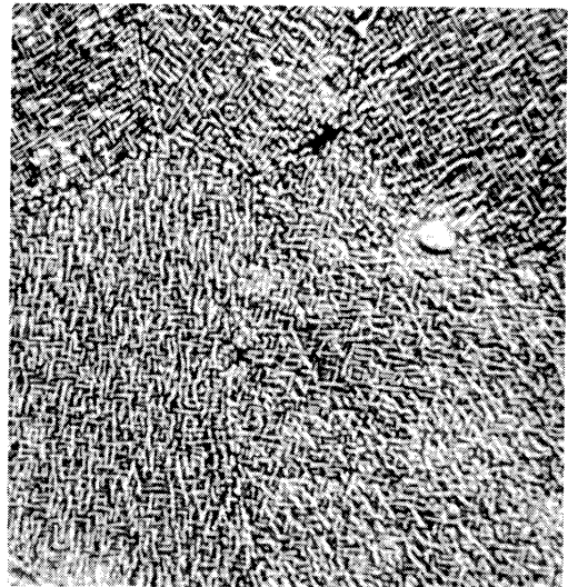
Fig. 2. MgO-Fe 2 O 3 microstructure. Example: 70 MgO-30 Fe 2 O 3 heated for 18 hours at 1600°C, quenched in water, reheated to 1100°C one hour. A Widmanstätten precipitate of magnesioferrite (bright) formed within the original single-phase magnesiowüstite. X 1000.
