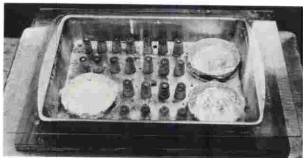
FIG. 2. Vapor substitution chamber used to prepare algae for mounting in a toluene based medium.
