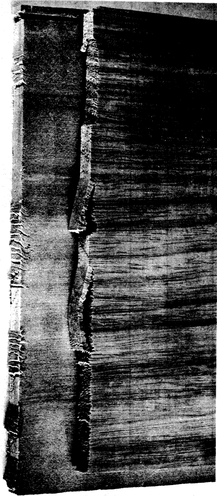
Fig. 21. Lateral vibration at 60 c. p. s. prevented type II failure and improved surface quality in cutting yellow-poplar (top) and common persimmon (bottom) at 0.5 in. per min. Vibration was alternately applied and removed. Cutting angle 25 deg., nominal chip thickness 0.030 in.
