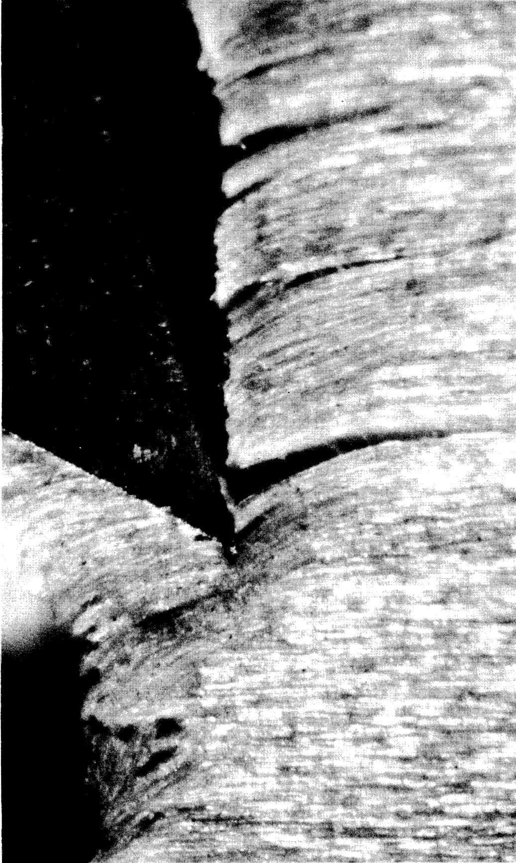
Fig. 11. Type I(b) failure in eastern white pine at 5 per cent moisture content. Cutting angle 30 deg., nominal chip thickness 0.030 in.
