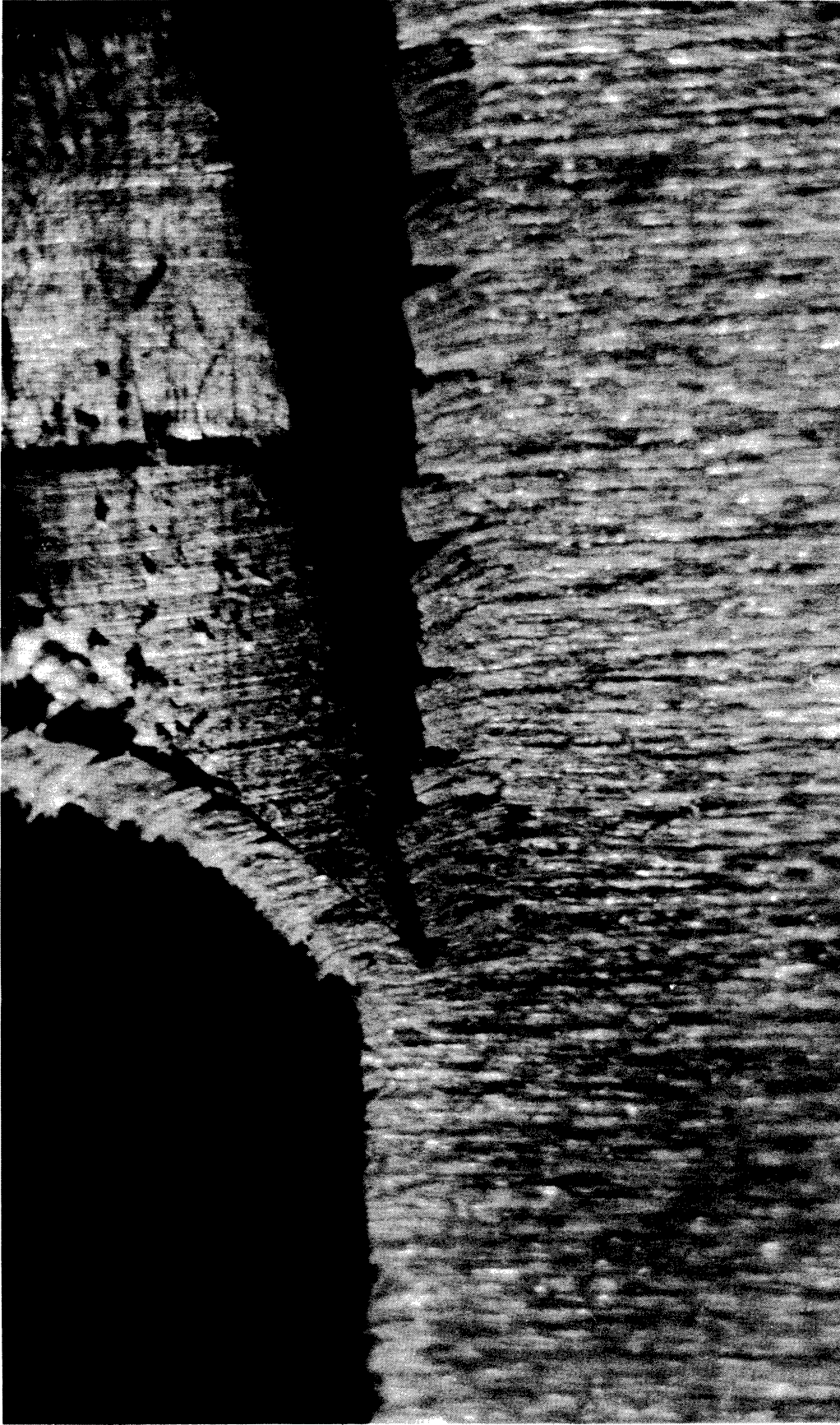
Fig. 12. Type II(a) failure in yellow-poplar at 5 per cent moisture content. Cutting angle 40 deg., nominal chip thickness 0.030 in. X10.
