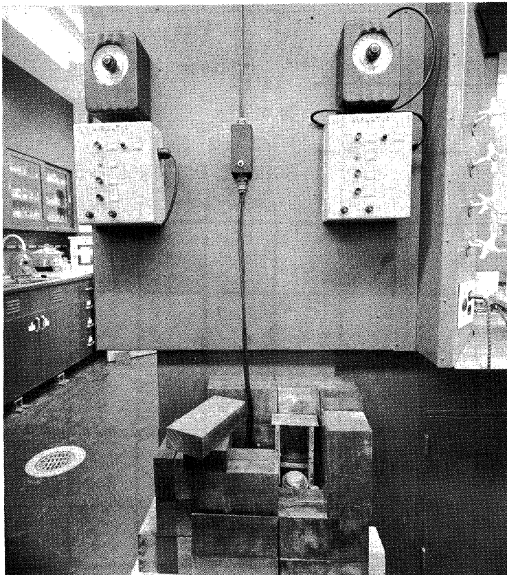
Figure 5. Gamma detector for 100-channel analyzer set up in hot lab next to hood.
