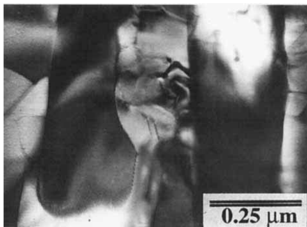
Fig. 10. TEM micrograph of the 30% \alpha' sample being hot-pressed at 1780^\circ\text{C} for 0.5 h.
