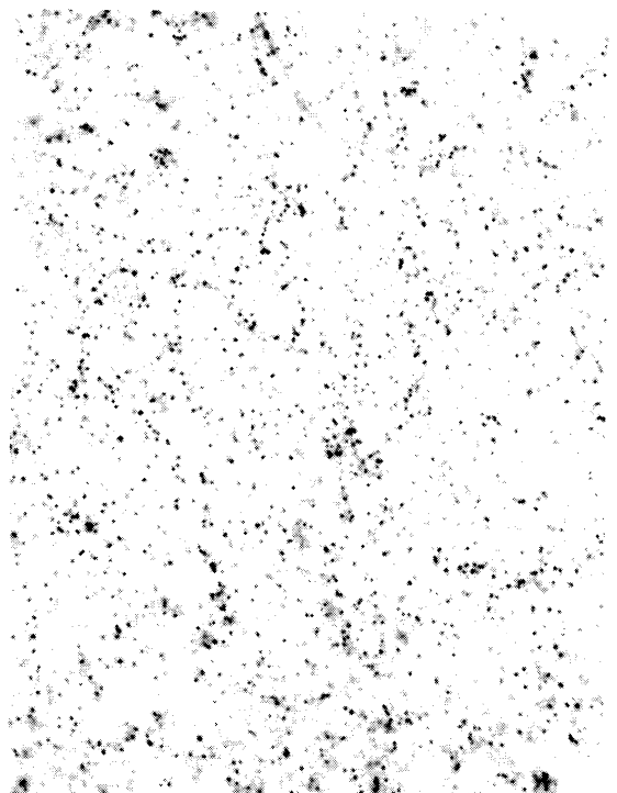
d) Tough Condition + Embrittled 100 Hours, 850°F, W.Q. Focus on Film
