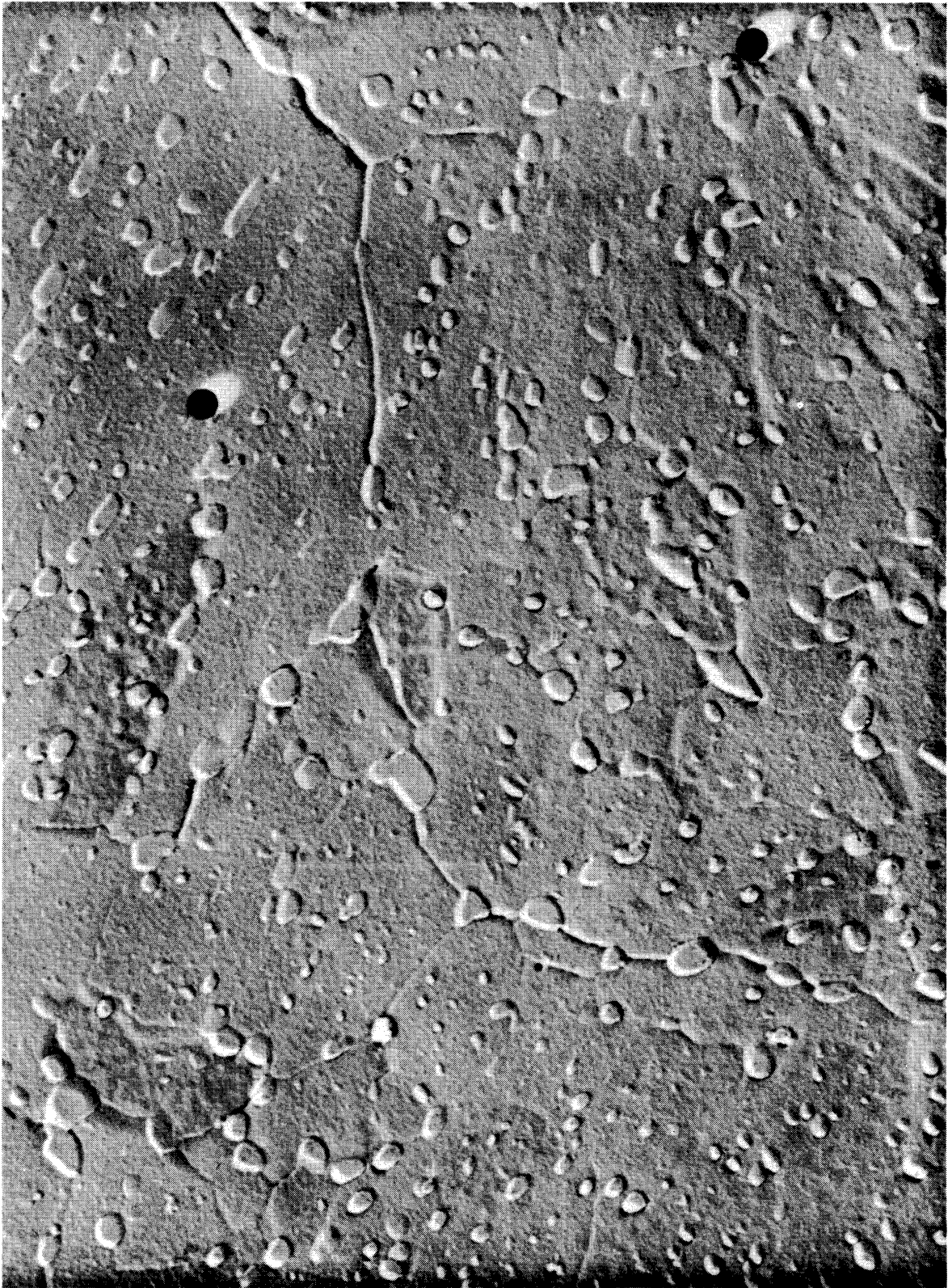
Figure 15. Electron Micrograph of Structure Produced by Embrittling Cycle of 100 Hours, 850°F, W.Q. Preceded by 1 Hour, 1250°F W.Q. Electrolytic Polish. Ethereal Picric Immersion Etch-10 Seconds. Magnification 20,000 x
