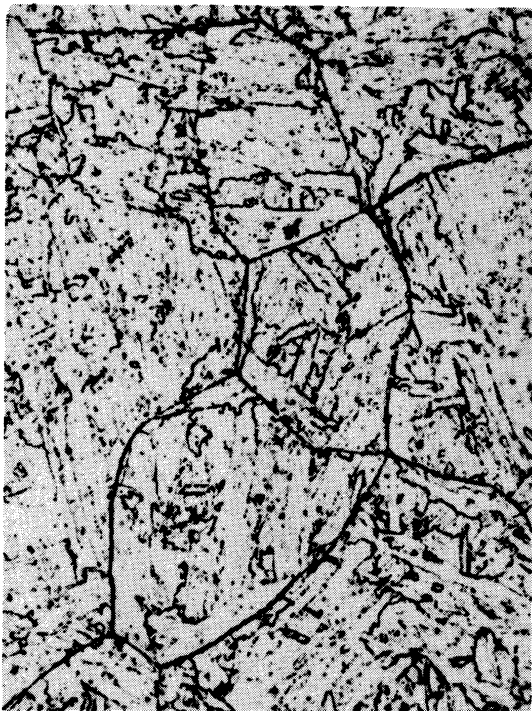
b) Tough Condition + Embrittled 500 Hours, 850°F, W. Q. Focus on Metal
