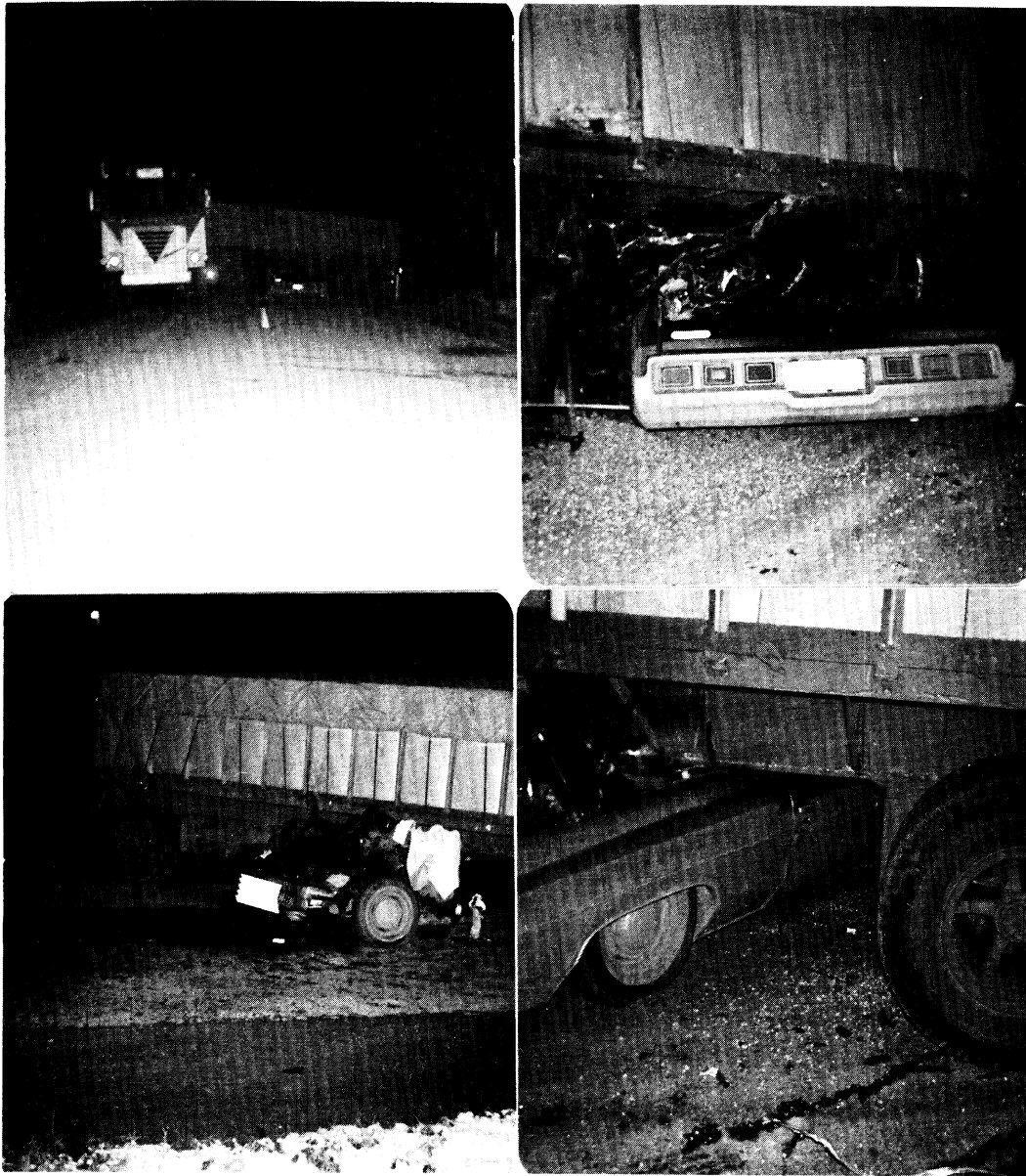
EXHIBIT C-3. A semi-trailer, stake body type, grain hauler, was astride both lanes of a 2-lane 2-way rural road at night (6:30 pm) while being backed into a private driveway. A passenger car (full size Chevrolet sedan), Eastbound on the same road completely underrode the trailer bed. The passenger car driver, a 20 year old male, who had not been drinking, was decapitated. Probable contributing factors were that the tractor, facing westbound with headlights on, appeared to be on-coming traffic, and thereby blinding the passenger car driver so that he did not see the non-illuminated side of the trailer. Estimated relative impact speed -45 mph.
