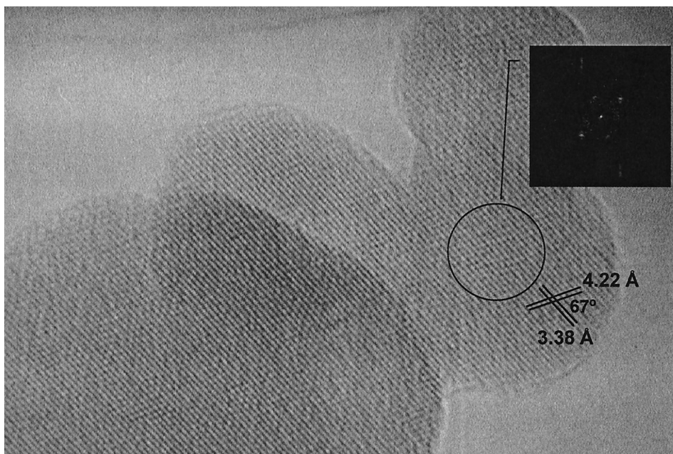
Fig. 10. HRTEM micrograph of as-processed mullite nanopowders (an SAD pattern is shown in the inset). All the particles have exactly the same orientation, suggesting that nucleation from one site leads to epitaxial crystallization.
