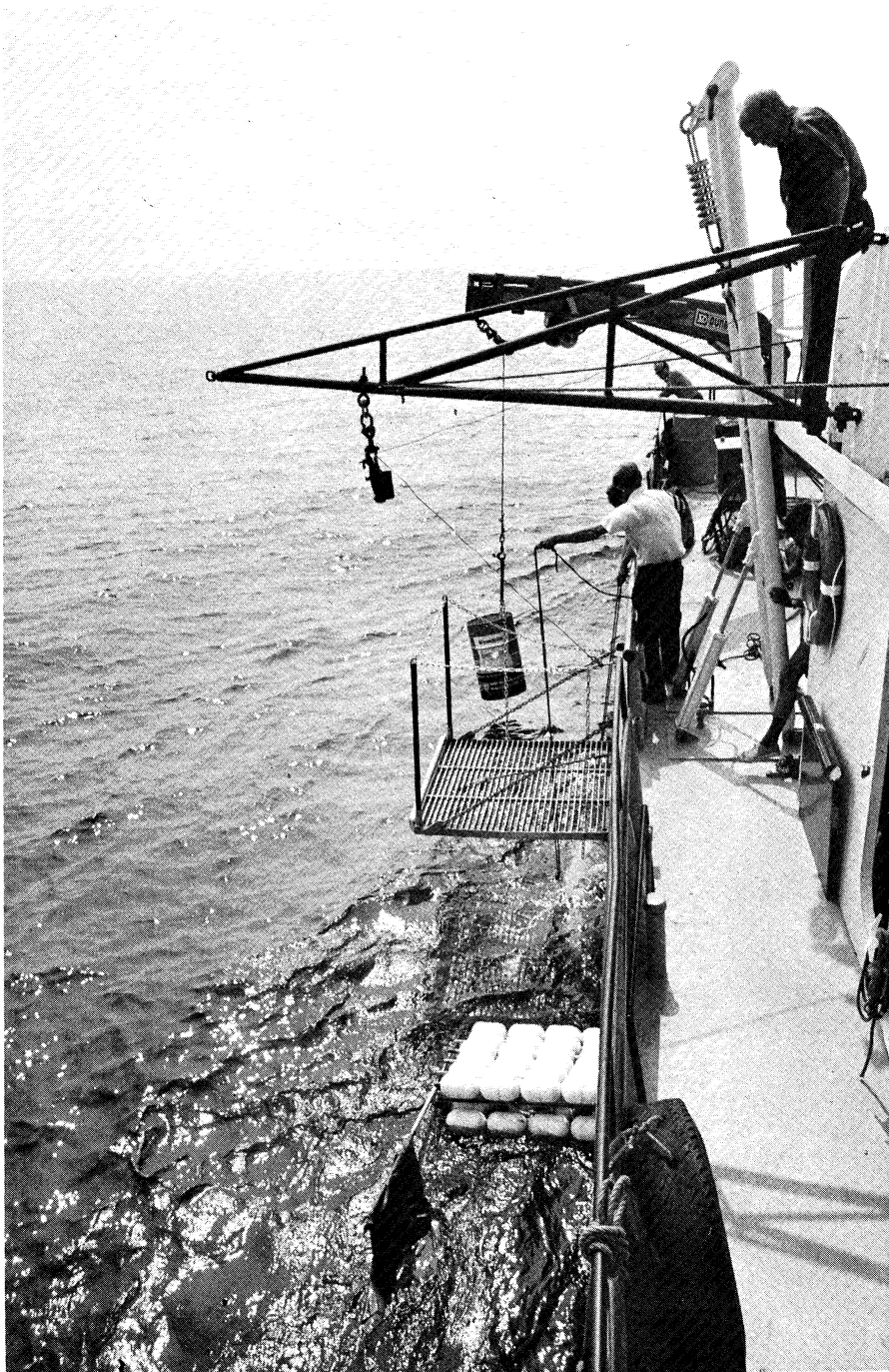
Figure 20: Sub-surface current meter mooring "R" being set from the starboard rail of the R/V LAURENTIAN on 9 August 1974, in the vicinity of Chicago, Illinois. In the foreground is the sub-surface (S.A.B.A.) buoy. Suspended above the lake surface is the barrel of concrete that acts as the anchor. Just visible beneath the surface is the E.G.&G. Model A102 current meter. (City of Chicago photograph).
