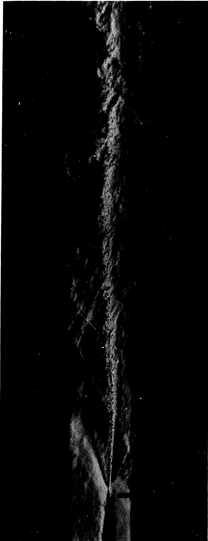
Figure 20. Schlieren Photograph of Supersonic Mixing.
