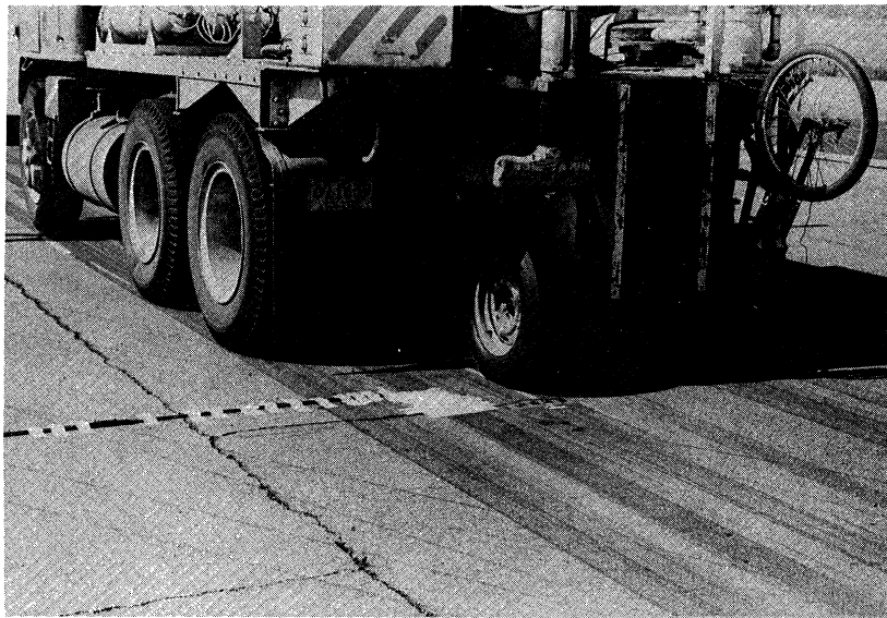
Figure 13. Treadless test tire mounted on truck.
