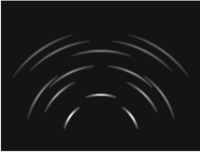
FIG. 6. Simulated RHEED pattern for rocksalt crystal lattice with (001) texture perpendicular to the plane of the film. Angular spread in texture is 15°.
