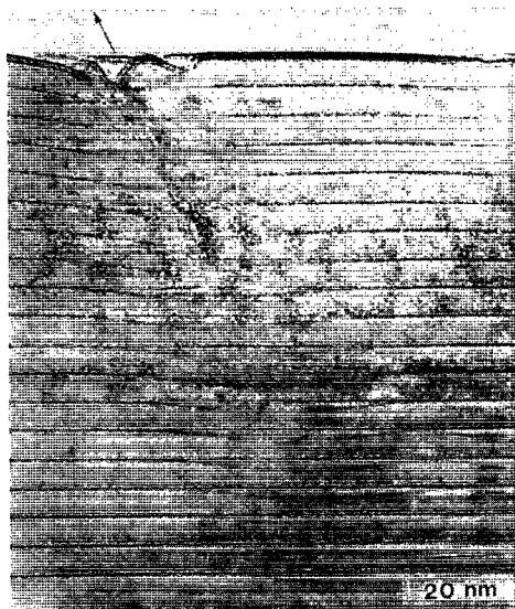
FIG. 1. Cross-section TEM image of a Si layer grown at 310 °C under "clean" UHV conditions (ambient hydrogen partial pressure). Ge marker layers (1/4 ML) show little change in surface roughness.
