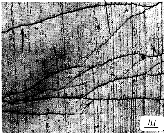
FIG. 6. (a) Pt-C surface replica of compression deformation bands in atactic polystyrene produced at 80°C at a nominal strain rate of 4 min -1 . Small arrows indicate a 500–1000-Å texture within the bands. (b) Pt-C surface replica of steps produced when deformation bands reach the back edge of the sample. Small arrow points to a step which has caused a slight displacement of the surface polish marks.
