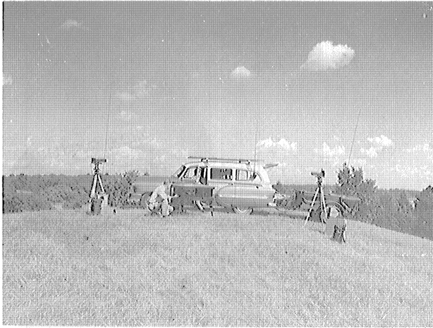
Fig. 9. The Mobile Receiving Unit. The Recording Polar Nephelometer and Portable Transmissometer are transported to the measurement site in a modified station wagon. A gasoline driven generator in the trailer furnishes electrical power for the instruments.
