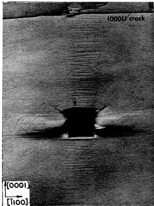
Figure 49. Slip traces around Vickers indentation (500 gm load) on the (11\bar{2}0) surface of MnTe. Oblique lighting. X150.
