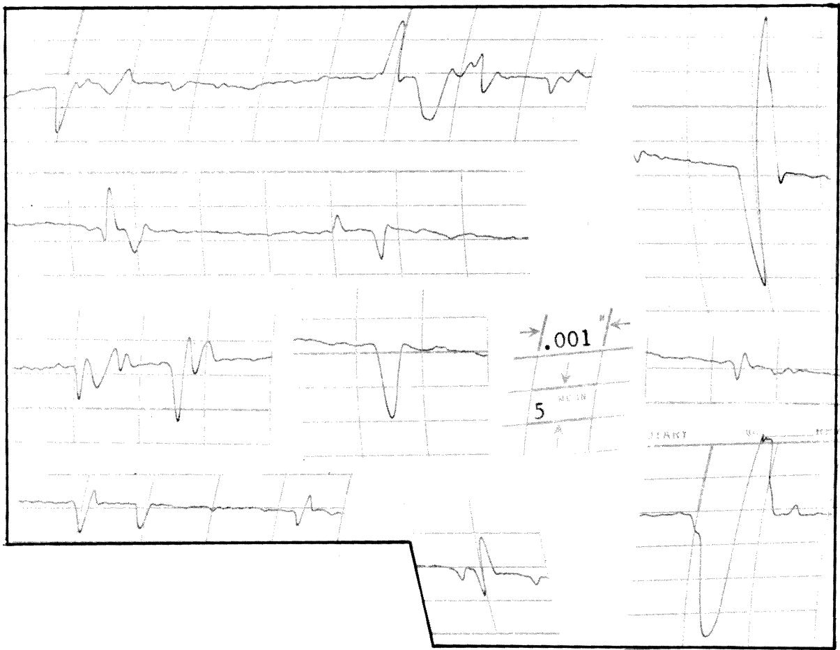
Fig. 85.--Typical photomicrographs and typical axial proficorder traces of cavitated surface of specimen No. 139-3 (304 SS) after 100 hours in water at a throat velocity of 200 ft./sec. for "standard cavitation" (a) nose area, (b) tail area.
