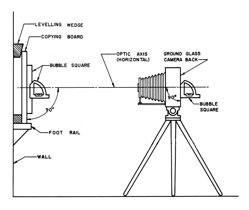
FIG. 2 ELEVATION VIEW
