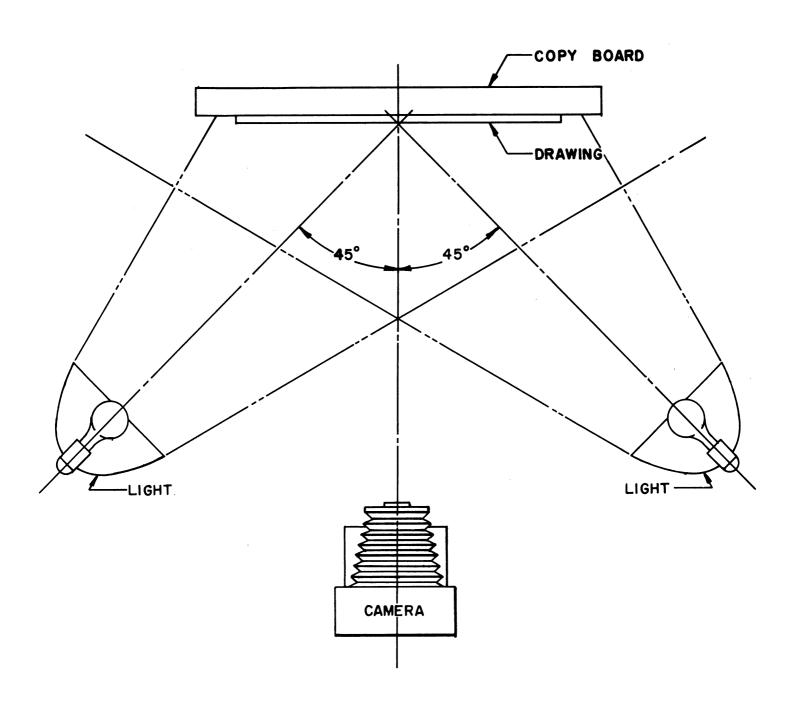
FIG. 3 PLAN VIEW SHOWING PLACEMENT OF LIGHTS
