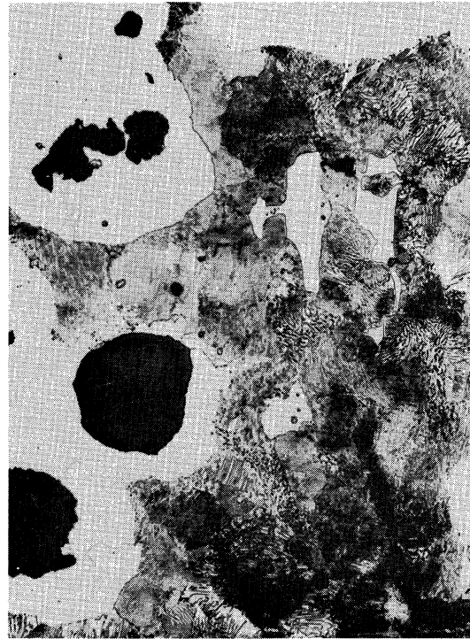
No Alloy - As-Cast Pearlite & Ferrite Matrix - 217 BHN
