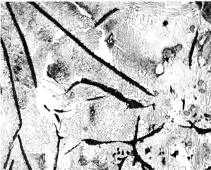
No Alloy Pearlite & Ferrite in Matrix
