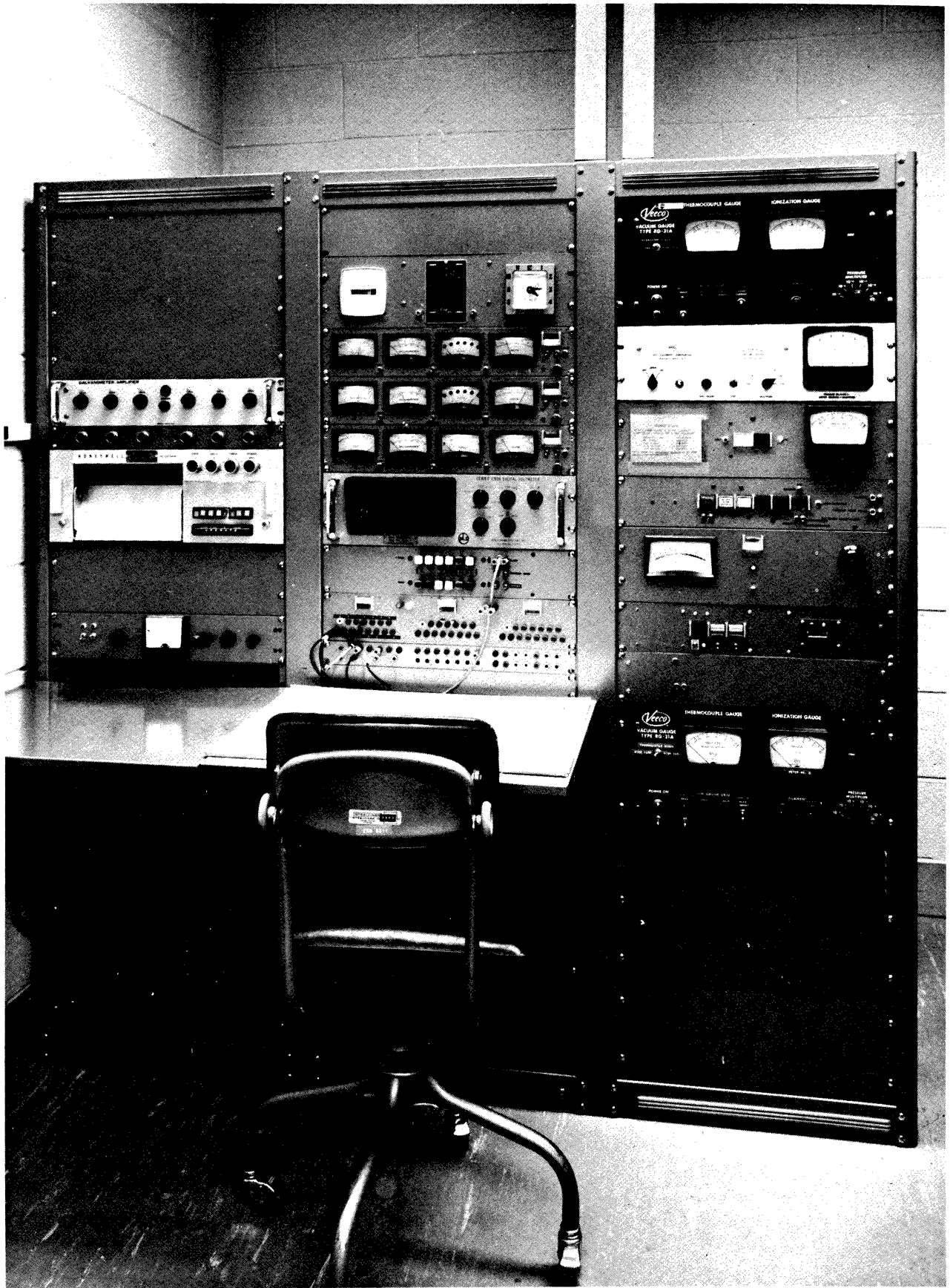
Fig. 58. Pressure calibration system--front view of control panel.
