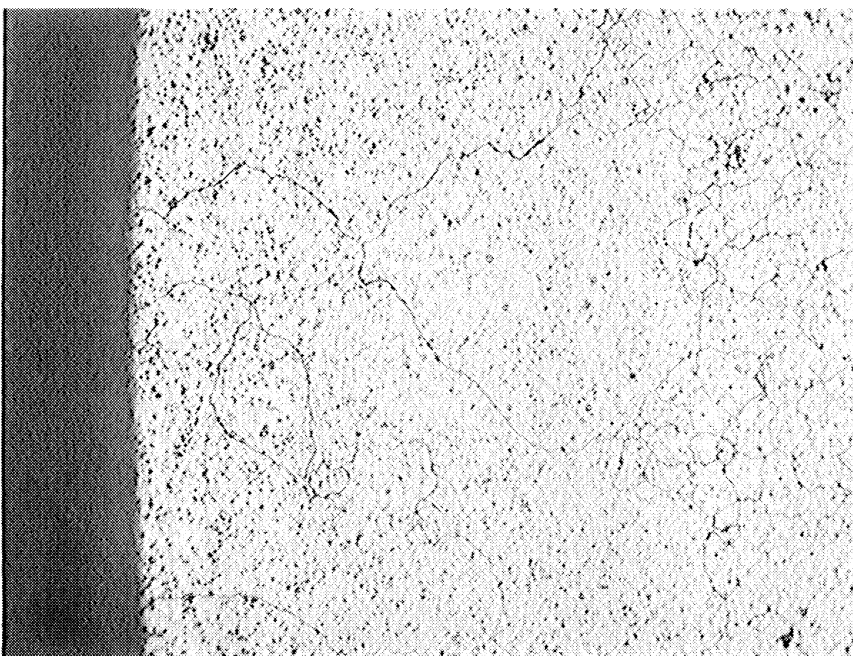
(c) Heated to 2150° F and air-cooled three times and finally solution- treated at 2300° F.
