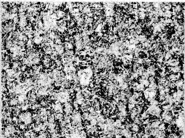
(c) Oil quenched 1900°F + tempered 4 hrs at 1200°F + creep tested 1003 hrs at 1100°F and 30,000 psi - 285 BHN.
