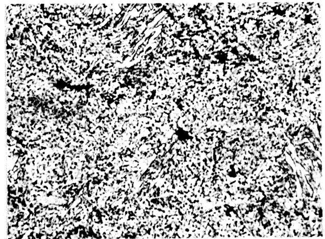
(b) 4340 Disk No. 3. Rupture tested 604 hrs at 1000°F and 20,000 psi - 238 BHN.
