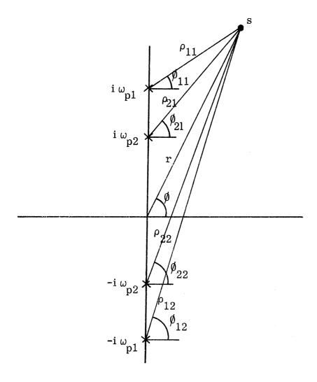
FIGURE B-1: POLAR REPRESENTATION OF  $s \pm i \omega_p$
