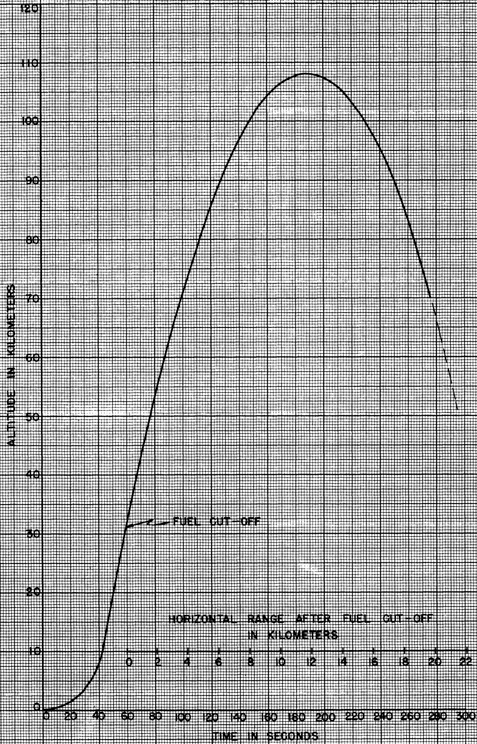
FIG. NO. A-8 ALTITUDE VS. TIME TRAJECTORY OF V-2 ROCKET NO. 20 FEB 20, 1947 BASED ON MASTER BEACON RADAR DATA
