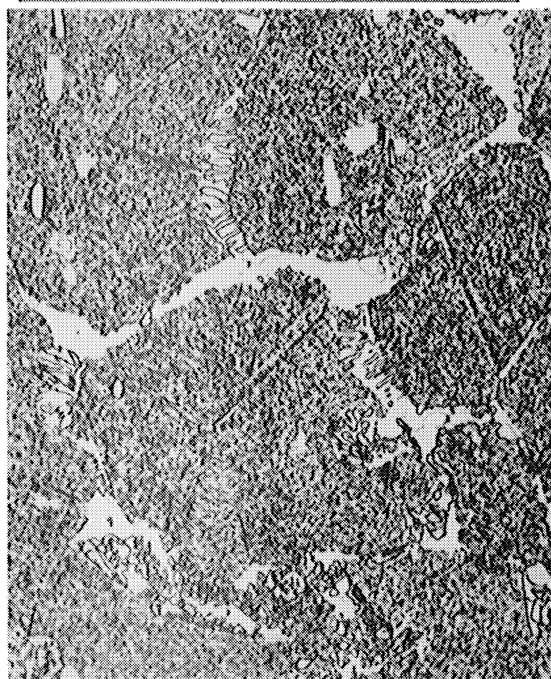
(b) Heat 1329B - 0.0070%S stress - 15,000 psi rupt. time - 927.6 hrs, RA - 48%
