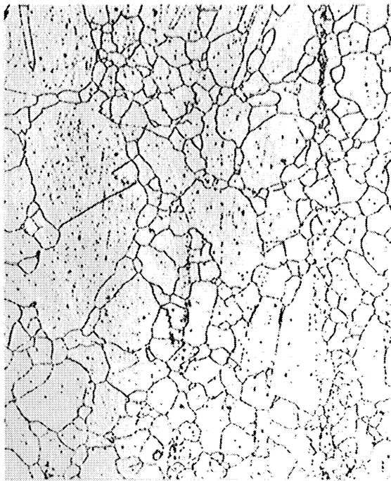
(a) Heat 1314A - 0.0049%S, no B and Zr added
