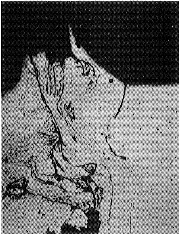
(b) stress - 2250 psi rupt. time - 31.9 hrs. RA - 3%
