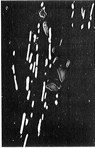
(b) Tau-Ti 4 C 2 S 2 , polarized
