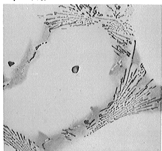
Figure 47. Influence of High Temperature Thermal Exposures on \text{Ti}_4\text{C}_2\text{S}_2 in the 20Cr-1.2Al-3.8Ti Alloy without and with Boron and Zirconium Added (1000X)
