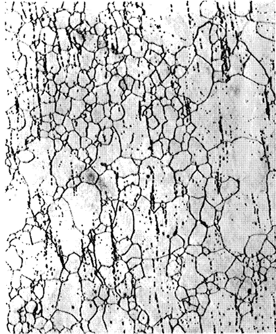
(b) Heat 1319B - 0.0640%S, 0.0035%B and 0.045%Zr added
