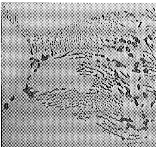
Figure 47. Influence of High Temperature Thermal Exposures on \text{Ti}_4\text{C}_2\text{S}_2 in the 20Cr-1.2Al-3.8Ti Alloy without and with Boron and Zirconium Added (1000X)
