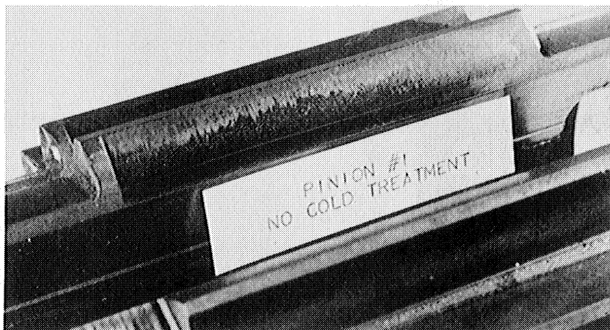
Fig. 5. Wear pattern after 10^6 cycles.
