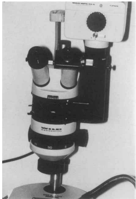
Figure 4. Measurements were made at a magnification of 50\times using a measuring eyepiece.
