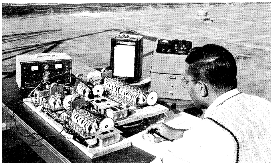
Fig. 3.16. Technician monitoring performance of timers and recording data during Graeco-Latin square experiment.
