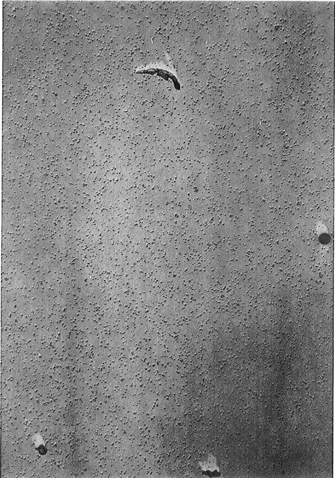
Figure 23. Photomicrograph of Collected Particles; 33,000X (Run 80514, 22.4 msec, p_c = 2259 psia, T_c = 2338^\circ\text{K} , f = 0.215 )
