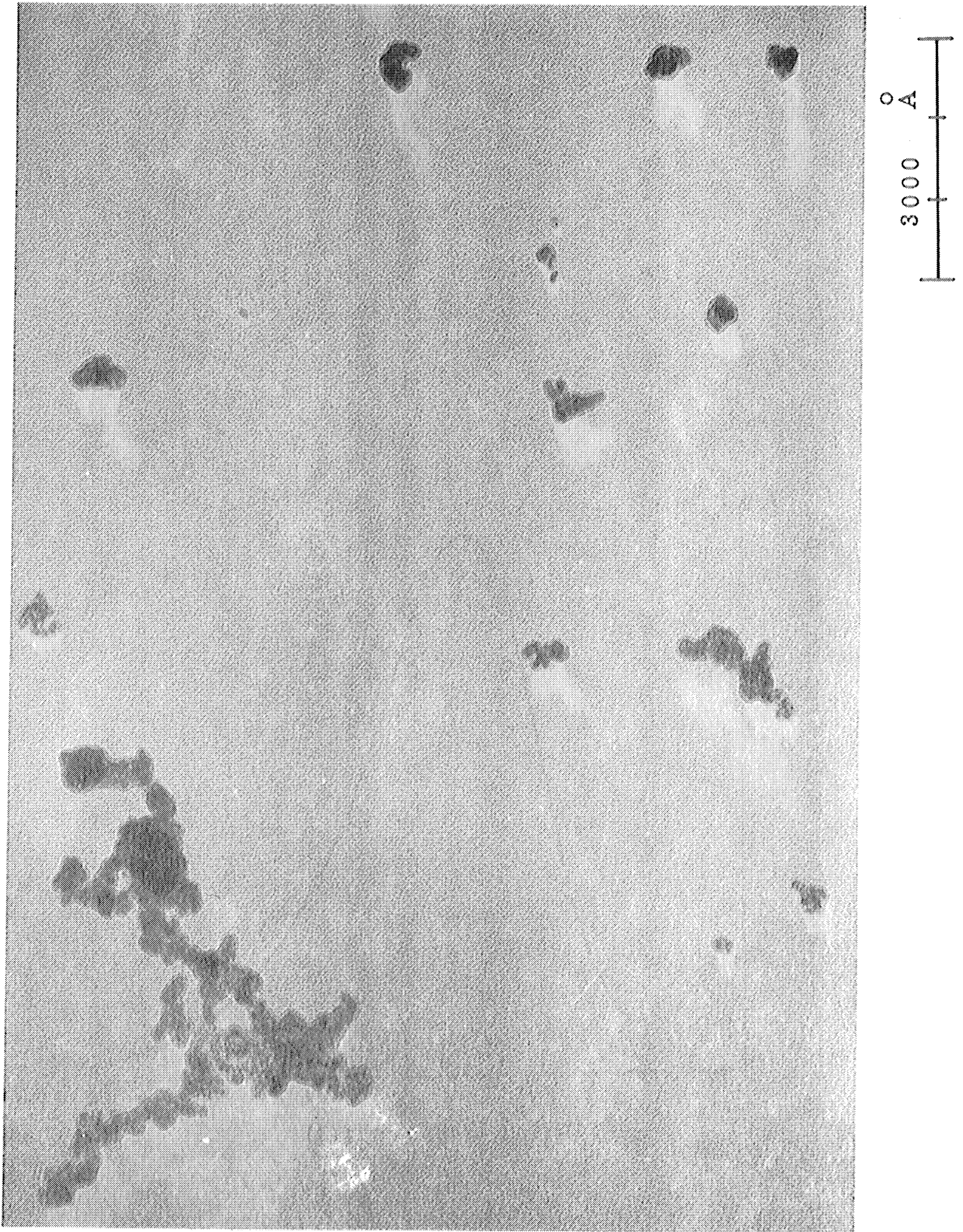
Figure 29. Photomicrograph of Particles Obtained Using the Mach 5 Nozzle; Sample Located Far Downstream of Nozzle Exit; 132,000X
