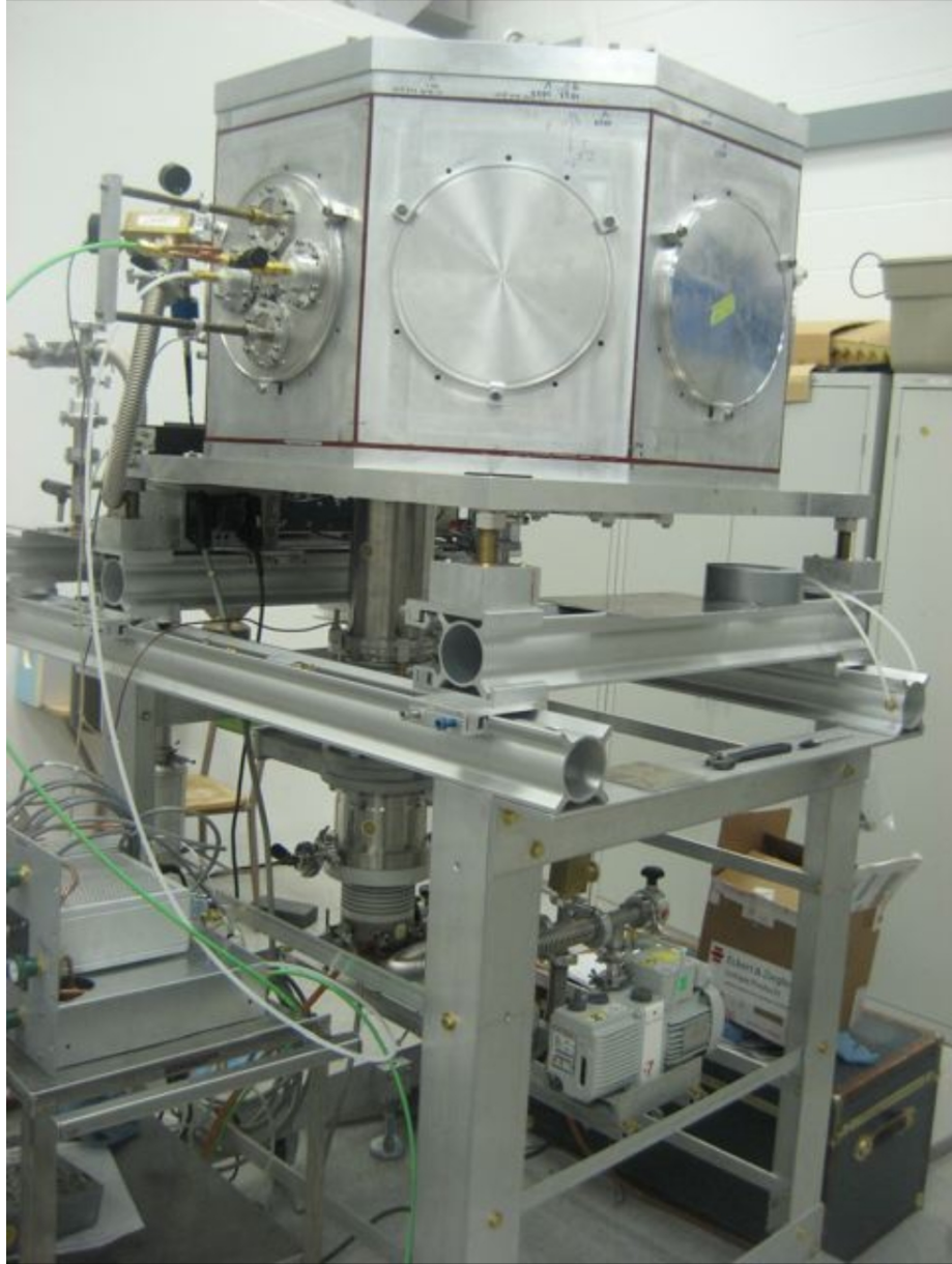
Figure 3.2: Picture of new ToF chamber constructed as part of this thesis project.
