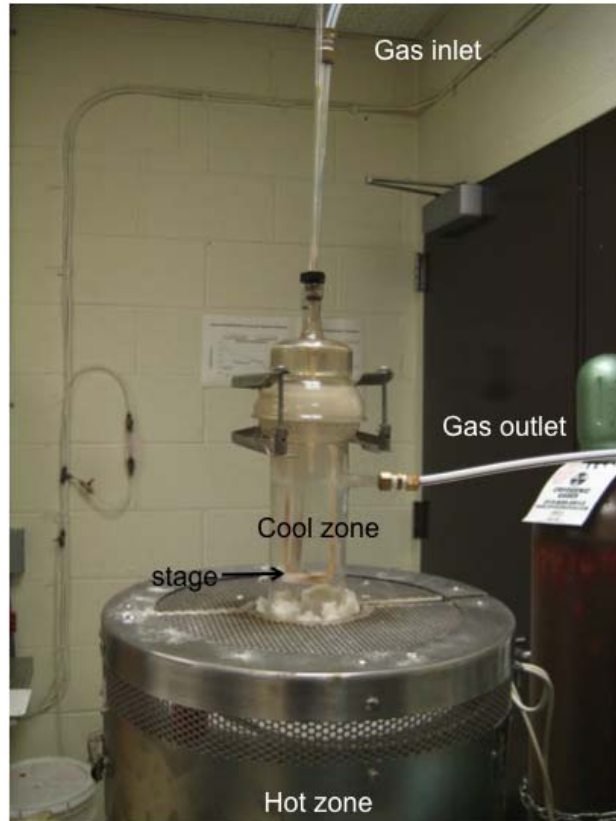
Figure 2.1: Photograph of custom made vertical tube furnace with a sealable quartz tube and movable stage.
