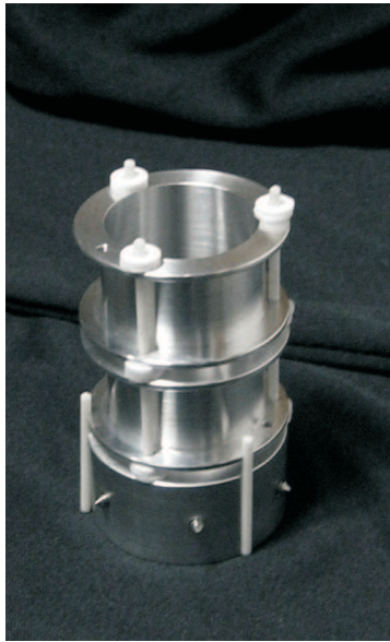
Figure 5.11: Ion lenses to control the ion path to the MCP.
