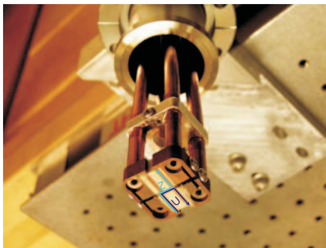
Figure 2.8: U and Z wires for the BEC magnetic traps.
